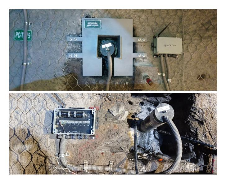
Geoteknik connected Ackcio VW Nodes (BEAM-VW-S8) to seven multipoint rod extensometers installed in the right and left axials of the tunnel along the mine's ore conveyor belt. They also installed three Ackcio Repeater Nodes (BEAM-RN) to ensure full data coverage. The Ackcio Gateway (BEAM-GW) at the surface was connected to the mine's ethernet, which shares the data with Ackcio's Snape software.
