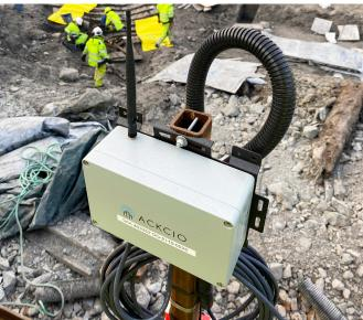
Cautus Geo's client wanted a reliable and efficient remote monitoring system. It chose Ackcio's wireless solution to eliminate the need to mount cables along the sheet pile to connect data loggers.
