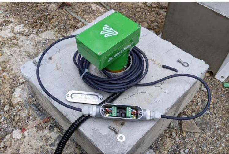
The sensor type – Measurand ShapeArrays – were proposed to replace conventional In-place inclinometers (IPI) for better data quality at three locations around the reservoir’s perimeter with a high risk of landslides. To get the data flowing reliably from the field, DECL chose Ackcio, with whom they have worked on two previous projects, for a few reasons.
