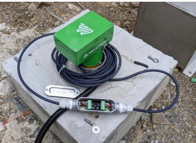
The sensor type – Measurand ShapeArrays – were proposed to replace conventional In-place inclinometers (IPI) for better data quality at three locations around the reservoir's perimeter with a high risk of landslides. To get the data flowing reliably from the field, DECL chose Ackcio, with whom they have worked on two previous projects, for a few reasons.
